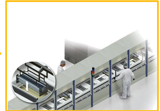
>> Wafers are etched, then a phosphorus layer and metal back surface are applied
