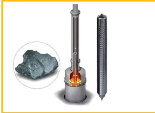
>> Raw silicon is melted down and grown into single crystal
